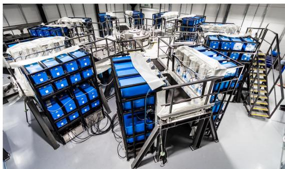
Fig. 7: M3, designed and built by First Light, uses extreme electromagnetic forces to launch projectiles at hypervelocities to test our fusion targets.
