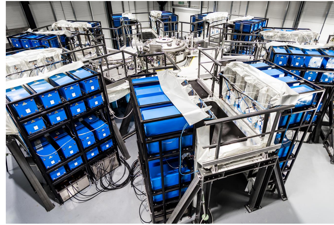
Fig. 1: Aerial view of M3 pulsed power generator
